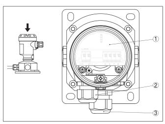
Fig. 28: Electronics and connection compartment
