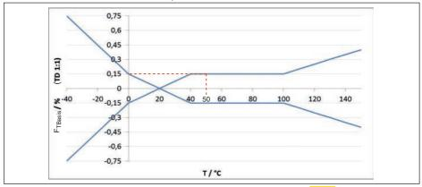
Fig. 42: Determination of the basic temperature error for the above example:  $F_{TRasic} = 0.15\%$
