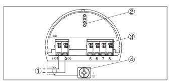
Fig. 25: Connection compartment - double chamber housing
