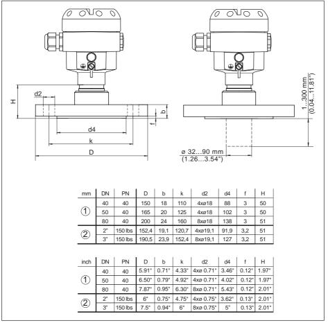
Fig. 53: CPT-2x, flange connection
