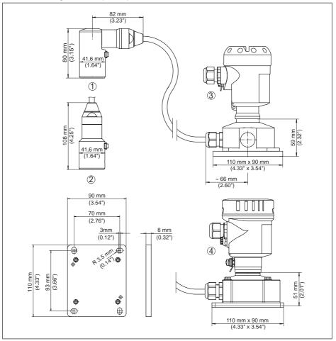
Fig. 49: IP68 version with external housing
