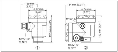
Fig. 43: Housing versions in protection IP66/IP67 (with integrated display and adjustment module the housing is 9 mm/0.35 in higher)
