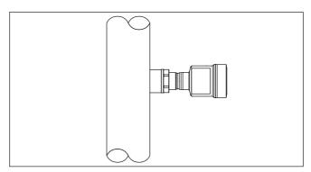
Fig. 2: Process pressure measurement CPT-2x
