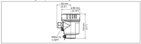
Fig. 48: Housing version with protection rating IP69K (with integrated display and adjustment module the housing is 9 mm/0.35 in higher)
