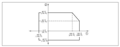
Fig. 40: Temperature derating CPT-2x, version up to +130 °C (+266 °F)
