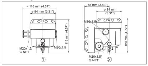
Fig. 44: Housing versions in protection IP66/IP67 (with integrated display and adjustment module the housing is 9 mm/0.35 in higher)
