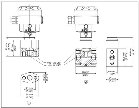
Fig. 55: CPT-2x, connection acc. to IEC 61518
