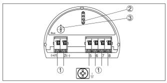
Fig. 22: Electronics compartment - double chamber housing
