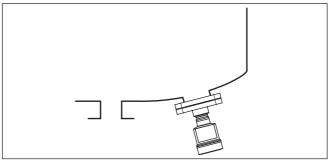
Fig. 18: Measurement setup for the level measurement
