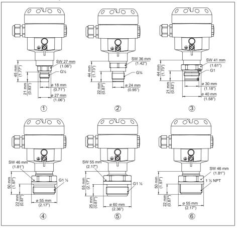
Fig. 51: CPT-2x, threaded fitting front-flush
