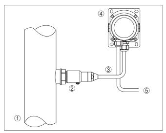
Fig. 19: Configuration, process module, external housing
