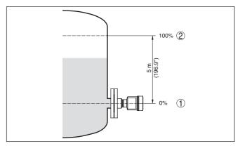
Fig. 34: Parameter adjustment example "Min./max. adjustment, level measurement"
