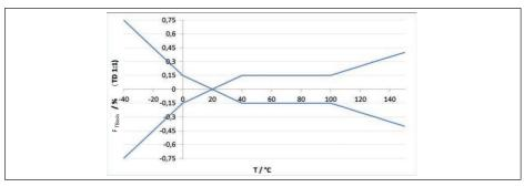
Fig. 39: Basic temperature error F<sub>TBasis</sub> at TD 1:1
