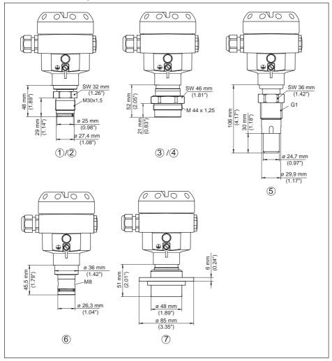
Fig. 54: CPT-2x, extension fitting
