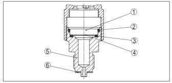
Fig. 4: Recessed installation of the measuring cell (example: manometer connection G1/2)
