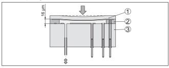
Fig. 3: Configuration of the ceramic measuring cell
