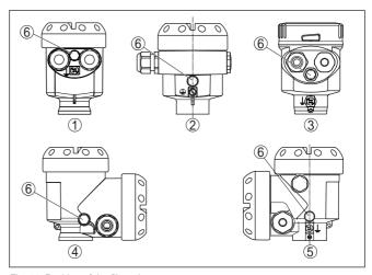
Fig. 11: Position of the filter element
