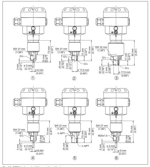
Fig. 50: CPT-2x, threaded fitting not front-flush
