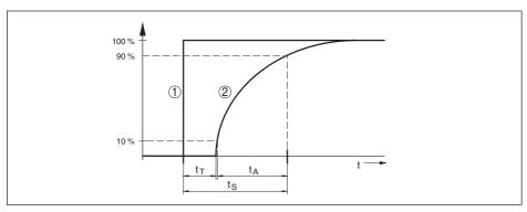
Fig. 38: Behaviour in case of sudden change of the process variable.  $t_{\tau}$  dead time;  $t_{s}$ : rise time;  $t_{s}$ : jump response time
