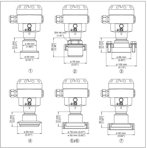
Fig. 52: CPT-2x, hygienic fitting
