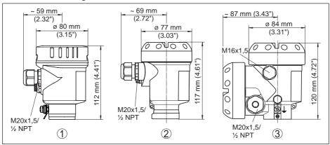
Fig. 46: Housing versions in protection IP66/IP67 (with integrated display and adjustment module the housing is 9 mm/0.35 in higher)
