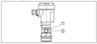
Fig. 12: Position of the filter element - Ex-d version
